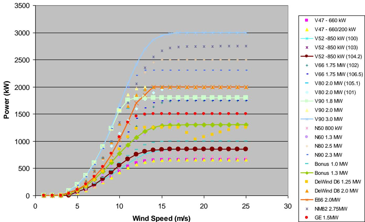
The figure below shows how much of the power is extracted at different wind speeds.
