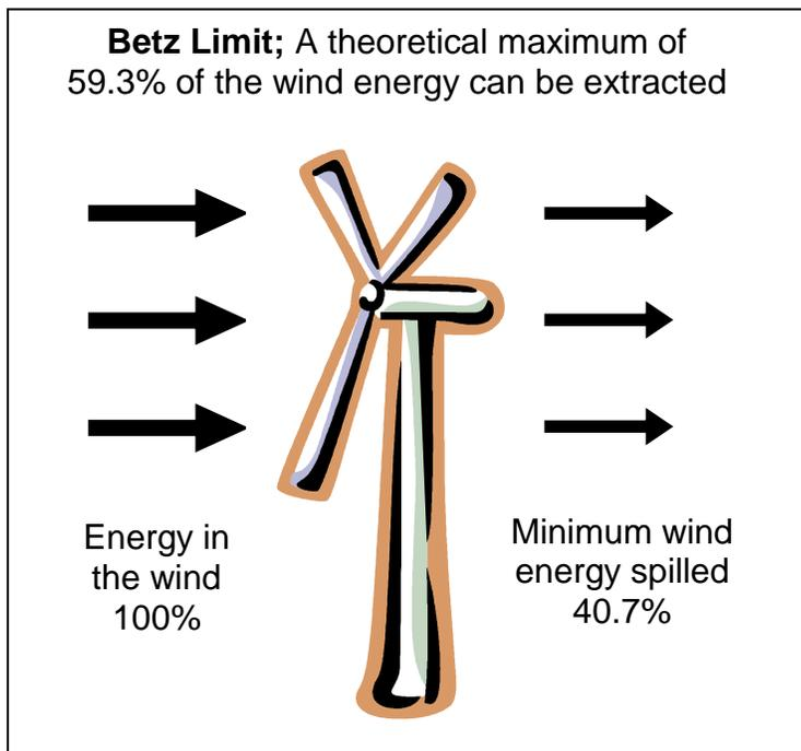
The Betz limit is an over estimate of the maximum energy extracted. British aerodynamicist Hermann Glauert's Blade Element Momentum Theory (1935) gives a lower theoretical maximum and more detailed models lower still. Practically, and under certain conditions, the most efficient modern turbine can extract close to 50% of the power in the wind after losses in a complete wind turbine system, including the blades, generator, bearings power conversion and transmission.
