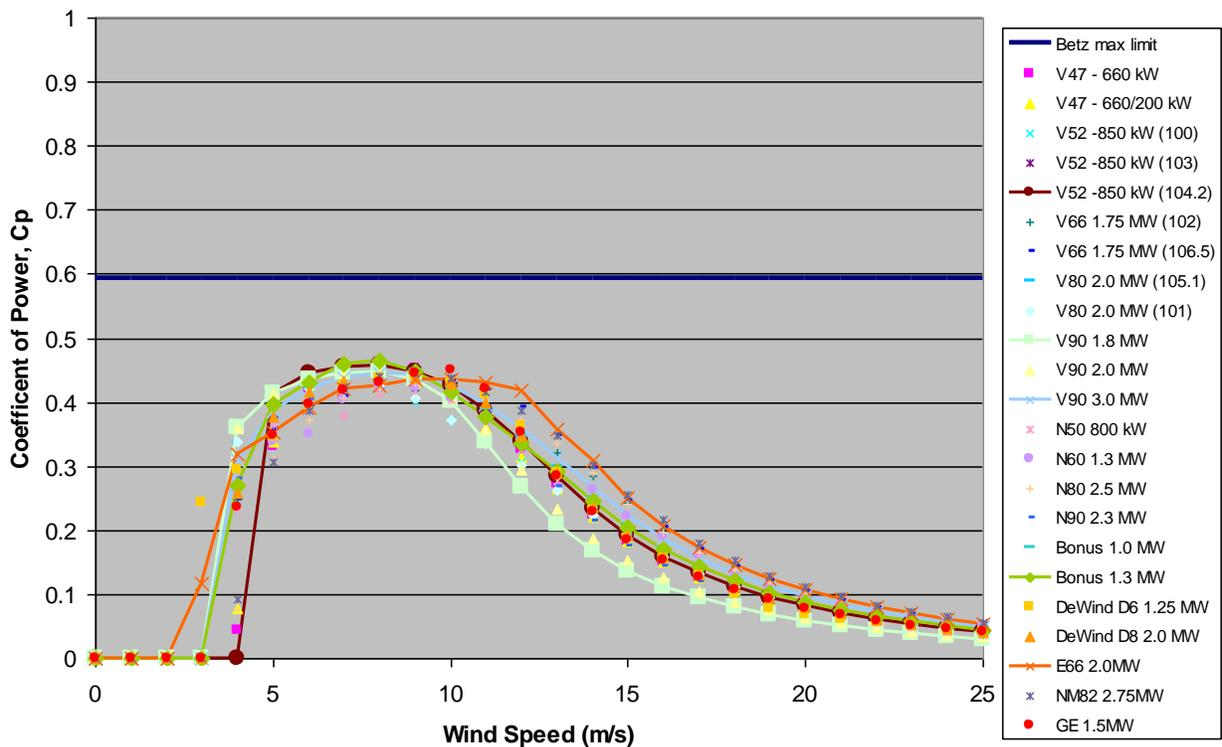
Once the engineering requirements of limiting the total output power for reasons of strength and durability, are included, the real limit is well below the theoretical limit and depends on the spread of wind speed seen at a specific site. Westmill's turbines extract about 32% of the energy in the wind passing through them in a year.
